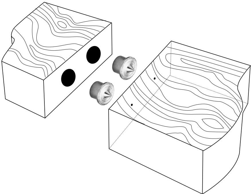
These dowel centers help to make it easy to precisely align the holes of two pieces of stock to be joined by a doweled joint—for example, a shelf and each of its supports. They can be used in conjunction with a dowel jig to show where the joining holes need to be drilled.
