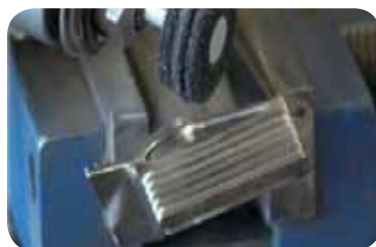
The non-woven fabric pressed in our VKS discs and shank tools can be profiled and thereby perfectly adapts to the geometry of the piece to be treated
