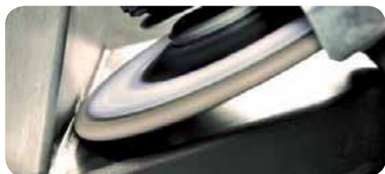
FS1 FUSION - Profiled grinding disc with a fine microsection comparable to a flap disc....
