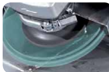
The LSZ F VISION provides with three clever recesses an unobstructed view of the workpiece
