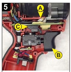
Be sure to tuck wire connectors into wire channel (A). Place trigger switch (B) and shuttle (C) into housing cavities.
