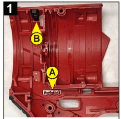
Insert fuel gauge light pipe (A) and mode select light pipe (B) into the slots on the handle.
