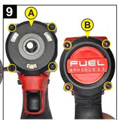
(A) Secure gearcase assembly to housing with four T-20 screws (fig.1).(B) Install rotor/back cap assembly and secure with four T-10 screws (fig.41).
