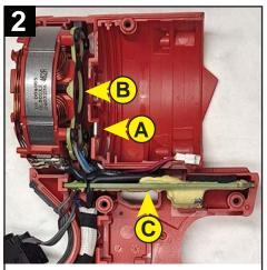
Place HV terminal wire clip on housing ridge (A). Insert electronics assembly into slots for stator (B) and PCBA board (C) into housing cavity as shown.
