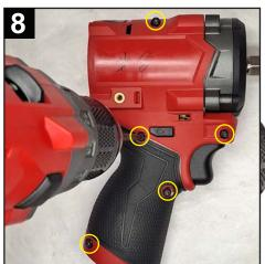
Carefully install right housing cover onto left housing support and secure with five housing halve T-10 screws (fig.41). Check functionality of shuttle and on-off switch.
