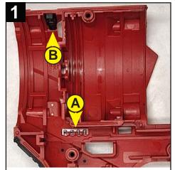
Insert fuel gauge light pipe (A) and mode select light pipe (B) into the slots on the handle.
